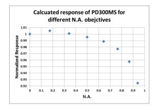
In practice the PD300-MS will work best when the focused light from the objective is centered on the active area of the sensor. This can be accomplished by first adjusting the system so that light is centered on the target on the backside of the sensor and then flip the sensor around for the measurement.
