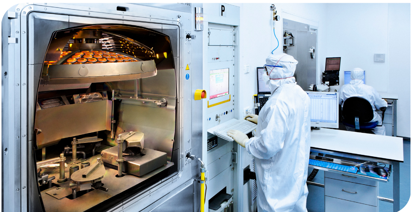
Figure 4: Ophir 1,000 clean room coating chambers
