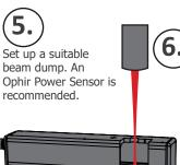
Center the beam in the BeamWatch Aperture.
