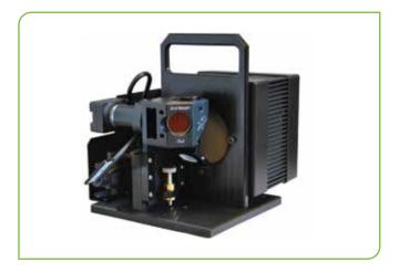
BeamCheck is an integrated laser measurement system designed to measure critical laser beam parameters for laser-based additive manufacturing systems BeamCheck includes a CCD camera for spatial measurements and a NIST traceable power sensor that will provide a complete analysis of the laser power density profile.
