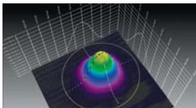
CO<sub>2</sub> laser beam prior to focusing optic
