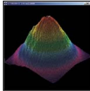
THz laser beam at 1.6THz (184 $\mu$ m).
