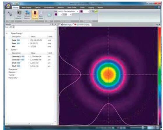
BeamGage recognizes the Pyrocam IIIHR & IV and allows you to quickly start analyzing your laser beam
