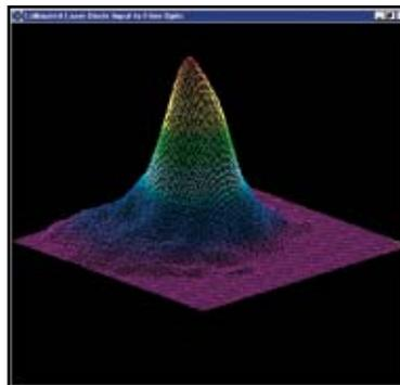
CO<sub>2</sub> laser with cavity misalignment.
