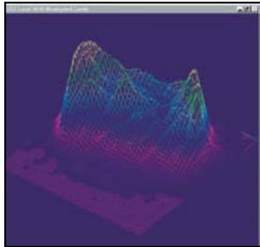
CO<sub>2</sub> laser with cavity misalignment.
