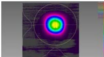
2D CO<sub>2</sub> laser beam prior to focusing optic
