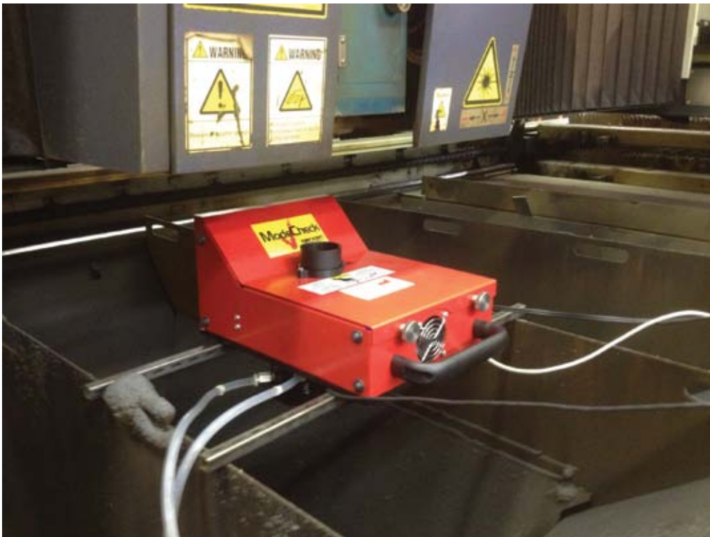
ModeCheck with optional MLA, profiling a CO 2 cutting laser with its processing head installed
